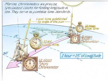
Illustrated above is the chronometer technique, used for navigating.
